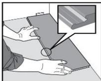
**Fig 1.** First plank, first row. Place a spacer of 12-15 mm thickness to the left and position the plank against the wall. Later, after 3 rows, you can easily position the flooring against the front wall with distances 12-15 mm.
