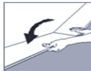
**Fig 2.** Second plank, first row tilt angle & place this plank gently and tight to the short end of the first one. Angle short end into place. Lengthways tap maybe required to secure tightly. **Please make sure both long edges and short ends are tight with no visible gaps.**
