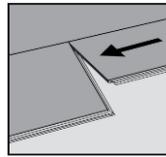
**Fig 8a** Second plank, second row place the panel at an angle into the groove of the previous row making sure that the end of the panel is near the short end of the previous panel. Lengthways tap will be required to flush and secure short end join.
