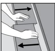
**Disassembling** Your floor can easily be disassembled, which enables replacement during installation and also after installation. Separate the whole row by carefully lifting up and slightly knocking just above the joint. Fold up or angle and release the whole long side. Disassemble the panels by sliding horizontally where possible or fold up and angle to release.
