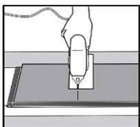
**Fig 5.** Cut with a jig saw – visual surface face turned down to eliminate/reduce damage to the face panel. Or if cutting using a hand saw, cut it with the visible face up. Then install it as previous plank.
