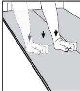
**Fig 8c** As it flattens itself to the floor press or gently tap the top of the short end of the installed panel until its flat. Finish installing this plank by tapping it with a tapping block on the long side to ensure secure installation.
