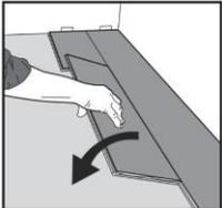
**Fig 8b** Tilt angle the panel down with a slight press to the left to the short end of the previous panel. Again using the tapping block tap it against the long end into the previous row. During the fold /angle down, make sure the panels are tight against each other.
