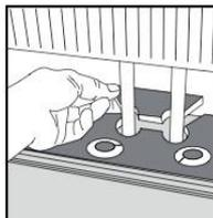
**Radiator pipes, installation at radiators.** Drill the holes 20 mm larger than the diameter of the pipes. Cut out the panel (with the thinnest blade possible) as per diagram. Install the plank as per normal. Glue the cut out piece back again.
