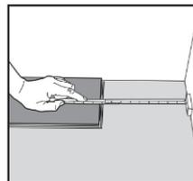
**Fig 4.** At the end of the first row, put a spacer 12 - 15 mm, to the wall and measure the length of the last plank to fit.
