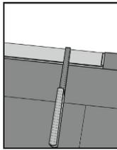
**Fig 10.** Last row (and perhaps also first row). **The Minimum width of the last plank should not be less than 50 mm.** Remember distance to wall is 12-15 mm. Tip! Put a spacer before measuring Cut the panels lengthwise and glue the short ends. See instructions below.
